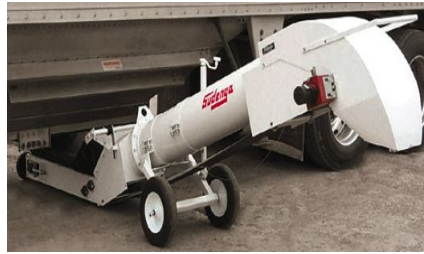
Belt Transfer Hopper
