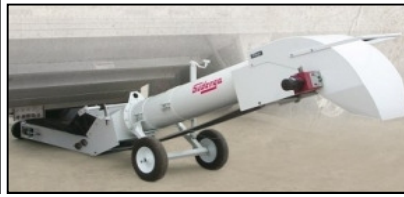
Belt Transfer Hopper
