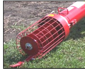
Oversize Intake, Double Flighting
