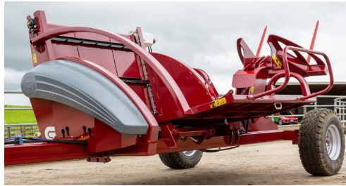
Easy Operating Hydraulic Tilt + Chain Outfeed
