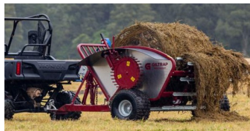
TPSI Bale Buggy feeder, trailed, ground drive (no PTO or hydr needed), for UTV or tractor
