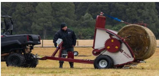
TPSI Bale Buggy feeder, trailed, ground drive (no PTO or hydr needed), for UTV or tractor
